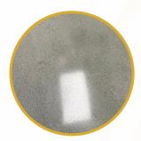
Polishable Concrete Overlays: Concrete overlays must be polished with 400 grit for minimum porosity with the installation of Coval Polished Concrete Sealer.
