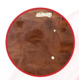
**Epoxy:** The spray down application of Coval UTC allows for more efficient installations over epoxy, providing superior abrasion and chemical resistance over urethanes and polyaspartics without the need for backrolling.
